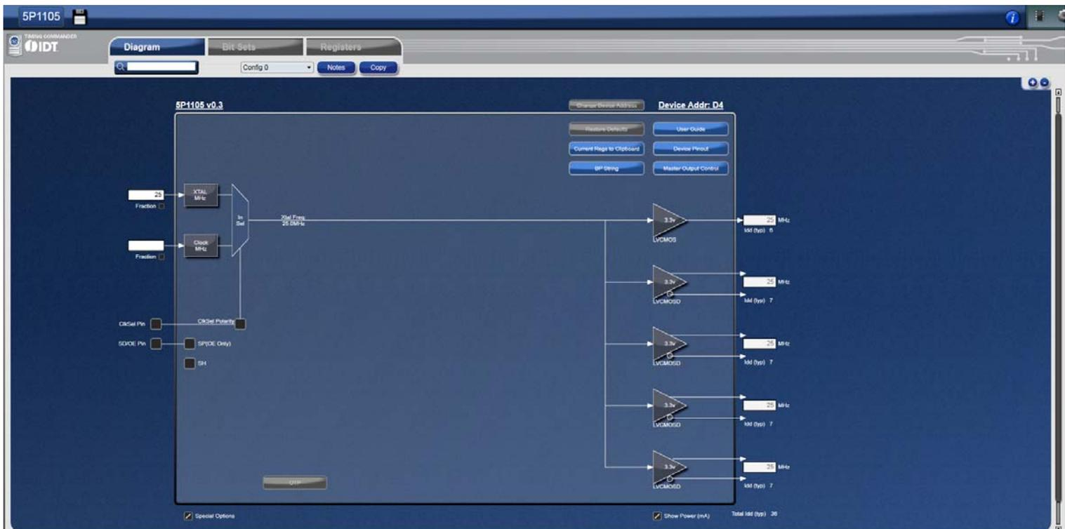
In the above configuration window, input source and frequencies can be selected and entered. Output frequencies can be entered. The GUI will automatically configure the PLL to generate desired outputs.
