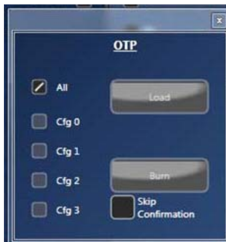
Figure 16. OTP Programming within Timing Commander GUI
