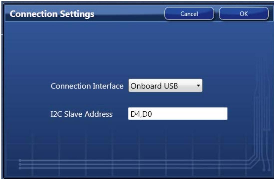
Use the default values in Connection Settings window and click OK to close it. Then click the chip symbol in the corner to bring out read/write command. When the connection is functioning, the area will turn green with “read” or “write” indicators. Please see Figure 14 below. The arrow pointing out of the chip means “reading from the chip”; the arrow pointing into the chip means “writing in the chip”.
