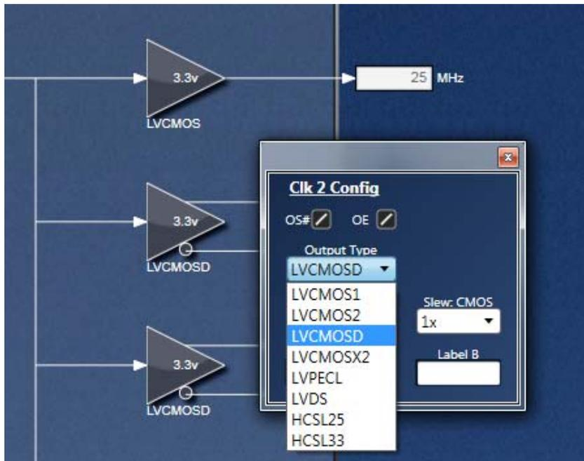
Clicking on the triangle box brings about output frequency configurations: Output type, Slew rate, Output voltage and Skew.
