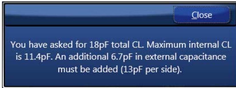
The user can still select the caps if the X1=X2 box is not checked. The Xtal CL then will be calculated automatically (Figure 6b.). Different values of X1 and X2 can be individually selected, although in almost all applications, an equal amount of capacitance for X1 and X2 ( $X1 = X2$ ) is recommended.
