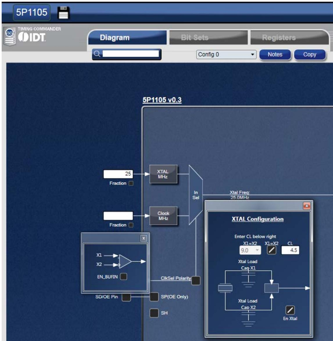
There are situations where both crystal and CLK are used as input sources. In this case, check both "En Xtal" and "EN\_BUFIN". Then use CLKSEL pin to select crystal or CLK source to be used as the input reference. The Truth Table is listed in Table 1 below.
