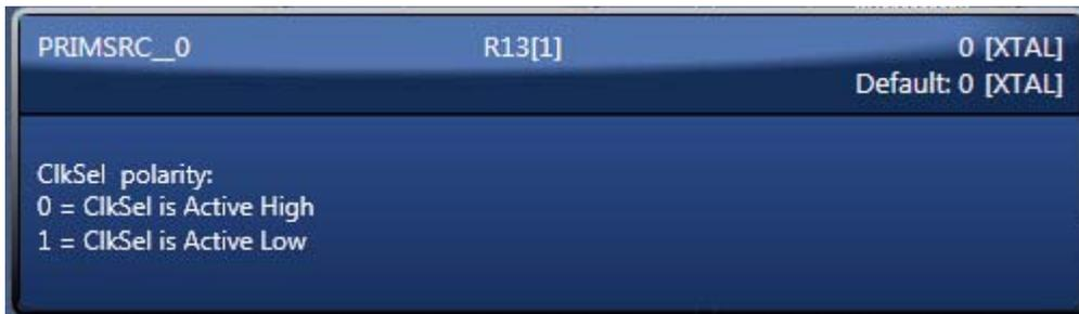
The CLKSel Polarity check box needs to be checked if using the CLK is selected as primary source and if CLK sel pin low like in Figure 5b. The timing commander will display the selected source based on the selection.
