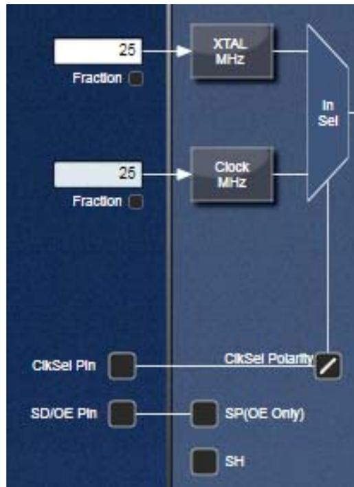
**Input Frequency Fraction box-** Input clock can be entered as a fraction if fraction box is checked and Fraction word is clicked as shown in Figure 5c below.
