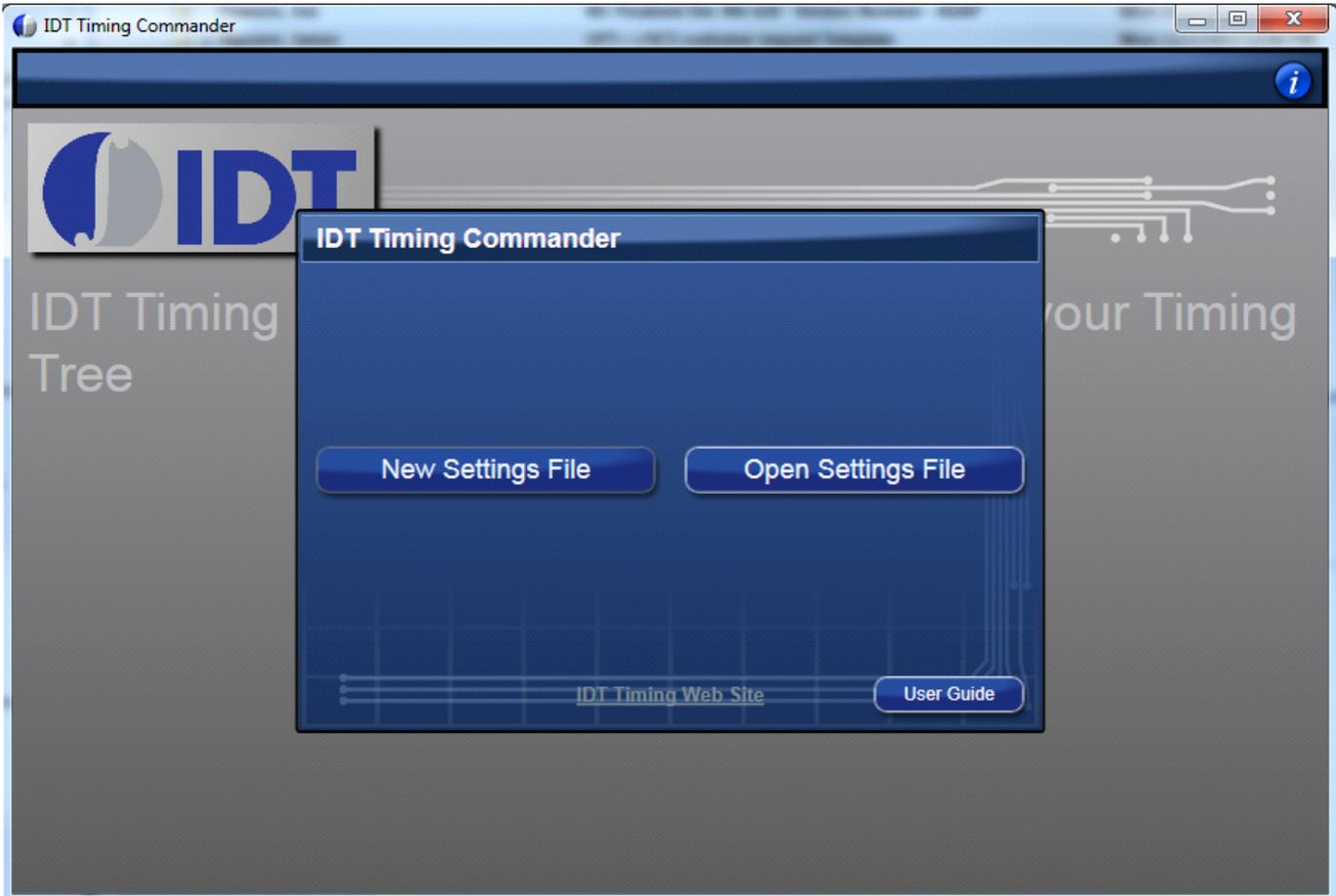
A settings file (.tcs) is a text file where the device input and output requirements are stored. From this window, an existing setting file can be opened to restore a configuration, or a new setting file can be started.
