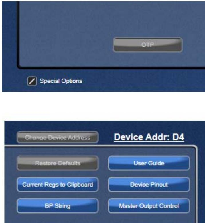
When connected to the device it is possible to change the I<sup>2</sup>C address by clicking on the **Change Device Address** button. This is permanent change that cannot be reversed.
