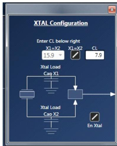
The max CL that can be created in the IC is 11.4pF. When entering a larger value, Timing Commander will display a window advising how much capacitance to add externally to each crystal pin to achieve the desired CL value (see Figure 6a below). TC is rounding the values to a integer value for the advisable external capacitors. Example for a XTAL CL of 18pF:
