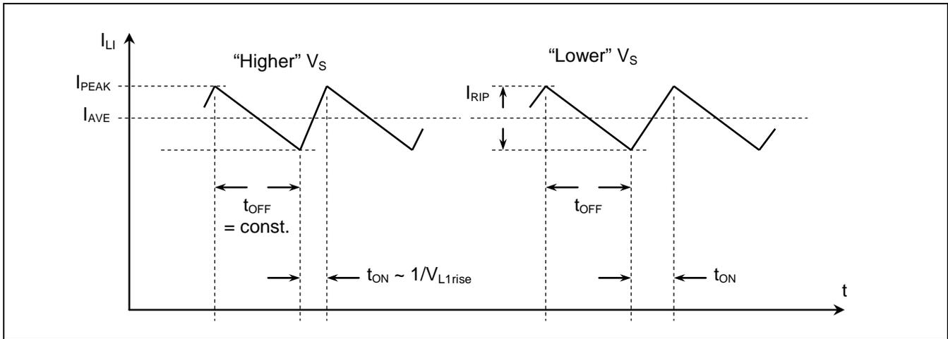
In a situation of constant average current, as shown in Figure 1.2, both rising and falling current changes  $\Delta I_{RISE}$  and  $\Delta I_{FALL}$ , defined as the current ripple  $I_{RIP}$ , must have the same amplitude. During  $t_{ON}$ † and  $t_{OFF}$ , the respective voltages across L1 are
