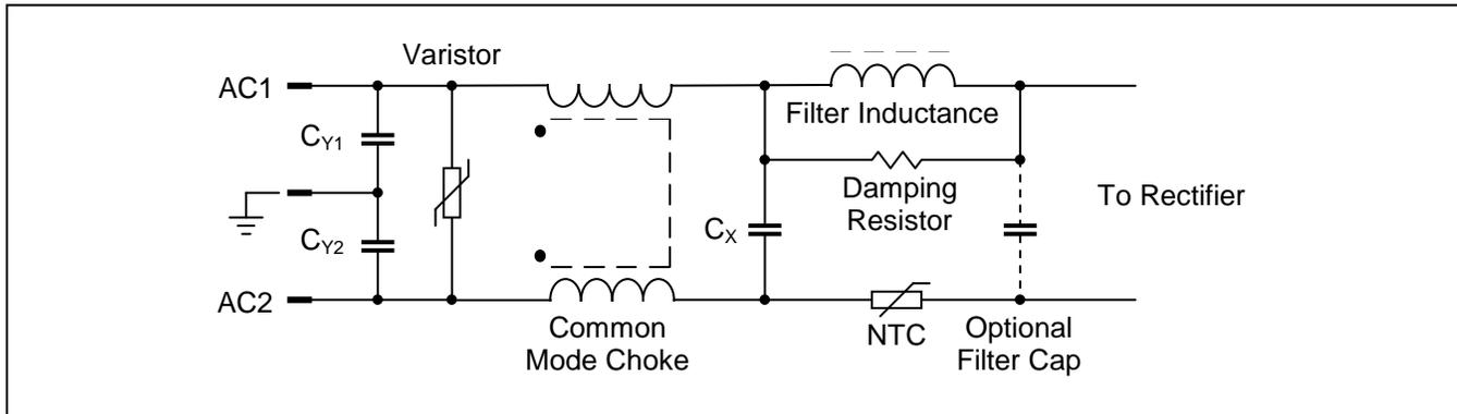
A varistor on the AC supply features over-voltage protection for the electronics, and a series NTC (negative temperature coefficient) resistor reduces inrush current when charging the bypass capacitor(s) after power on. Initially the NTC's resistance is high, and after being powered by the nominal supply current, it heats up and becomes low resistive.
