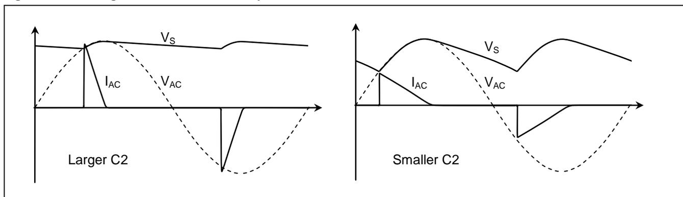
C2 must be large enough to sustain the maximum voltage of the LED chain until the AC amplitude is high enough to recharge it. Conversely, C2 should not be larger than necessary for a number of reasons:
