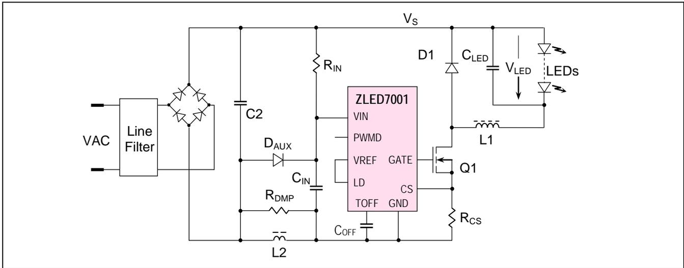
It is still necessary to power up the ZLED7001 from  $V_S$ ; e.g., via a series resistor, but this resistor must provide only the ZLED7001's current consumption, and  $V_S$  may be considered as the peak voltage at minimum  $V_{AC}$ , since  $C_2$  is not yet loaded by the LED current. Therefore under the worst case conditions,  $R_{IN}$  can be calculated as
