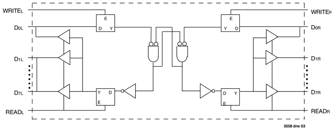
Figure 3. Simplified Diagram of One Semaphore Cell
