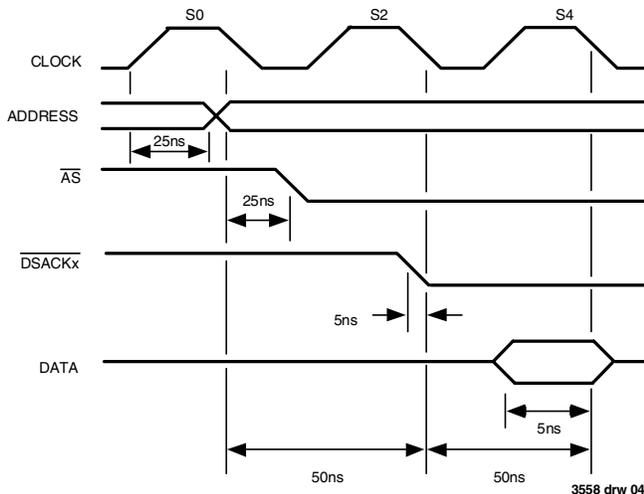
Figure 4. Read Cycle Timing for 20MHz 68020
