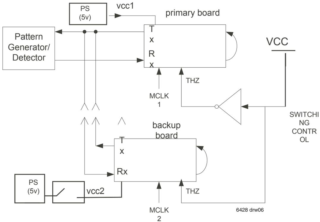
Figure 6. Test Setup #1 (Power Failure Test Setup)
