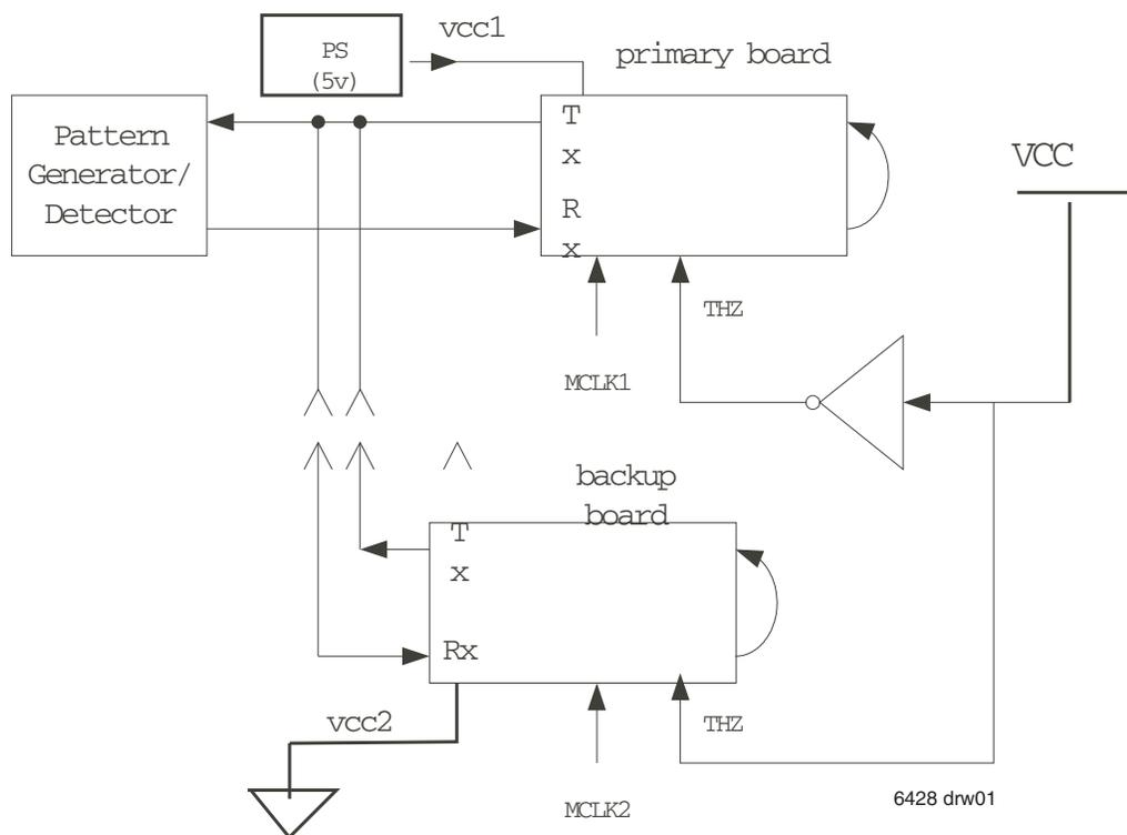
Figure 7. Test Setup #2 (Power Supply Short Test Setup)
