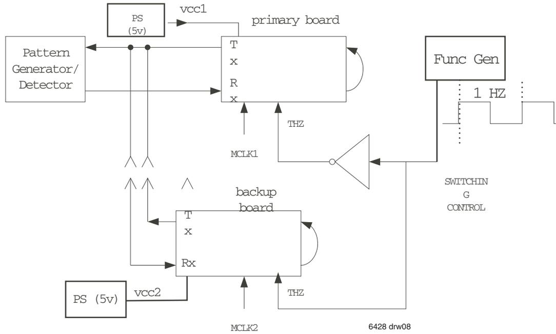
Figure 8. Test Setup #3 (Hot-Switch Test Setup)
