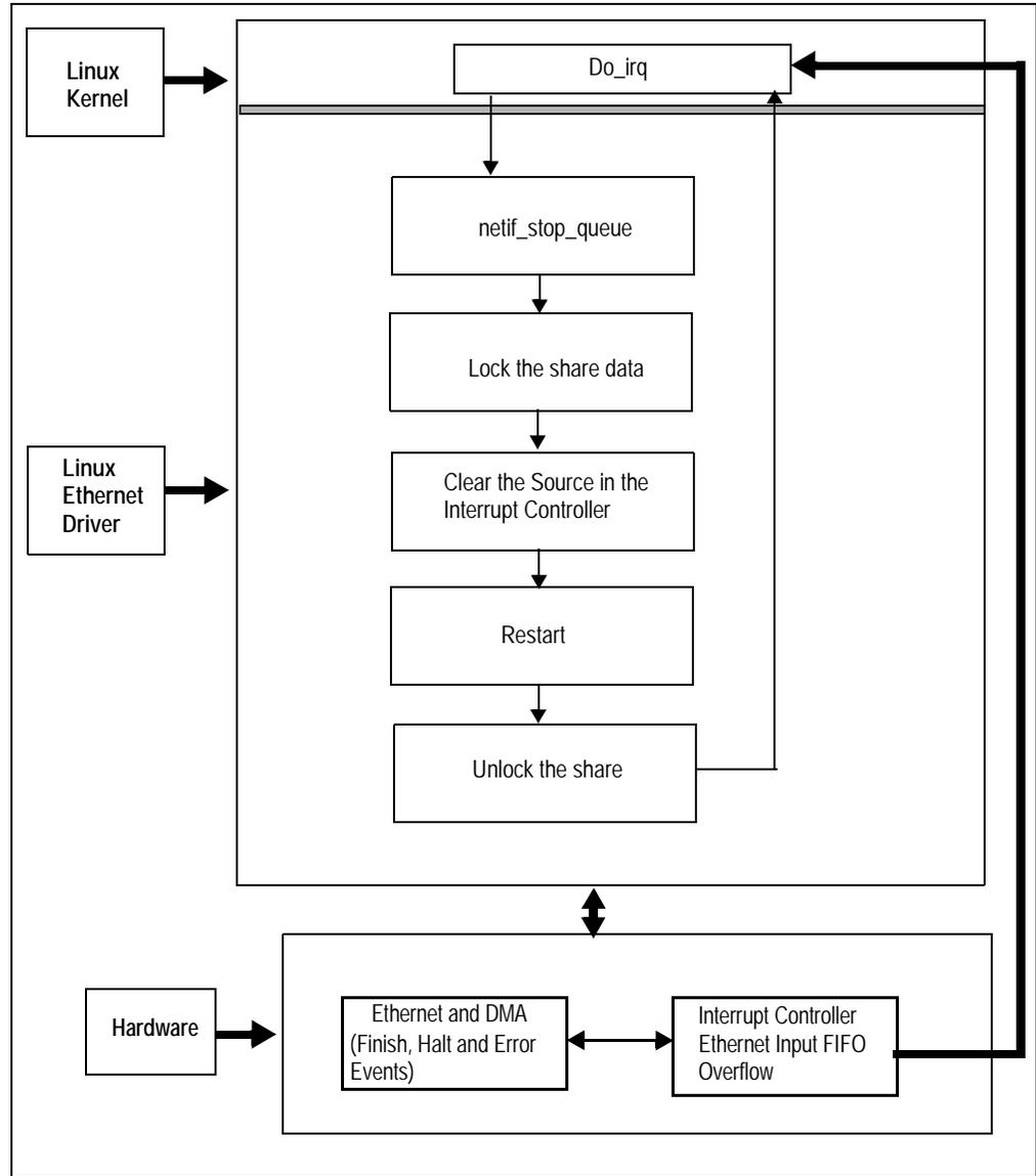
Figure 9 Receive Overflow Interrupt Flow Chart
