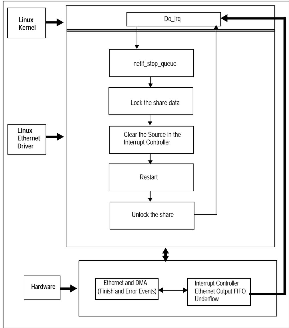
Figure 10 Transmit Underflow Interrupt Flow Chart
