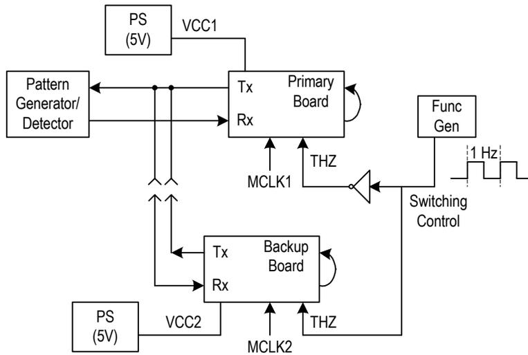
**Figure 9. Test Setup #2 (Hot-Switch Test Setup)**
