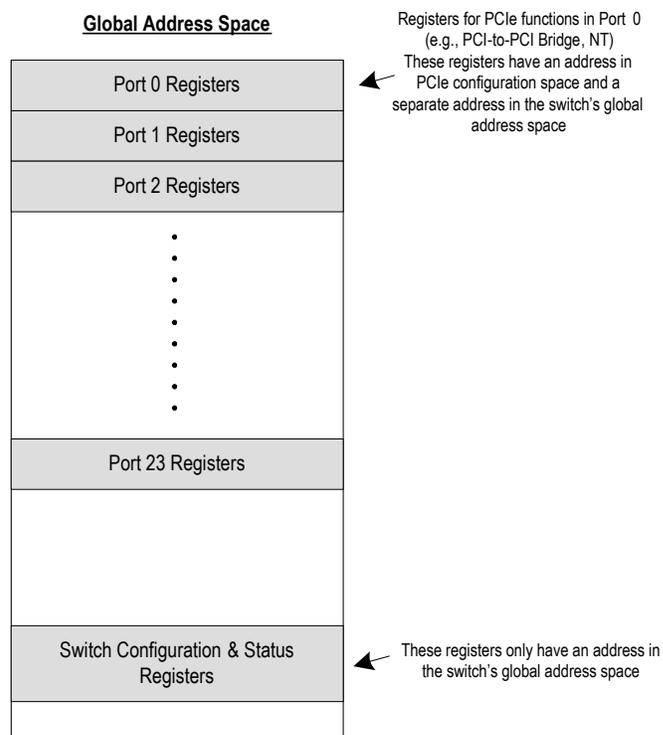
**Figure 2 Layout of the Switch's Global Address Space**
