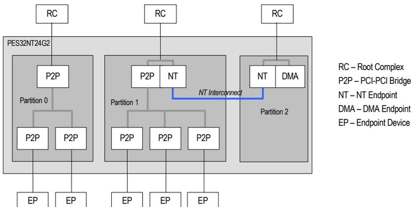
**Figure 1 The PES32NT24G2 Configured with 3 Switch Partitions**
