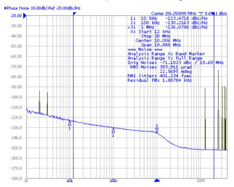
A few spurs appear above 30MHz but still no significant contribution to phase jitter or phase noise levels. This combination is perfect for the 5P49V6901 with four differential outputs.
