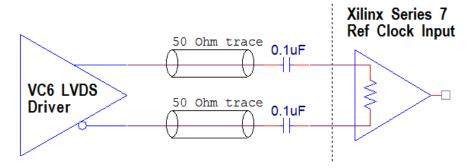
Only the AC coupling capacitors are needed to connect the VersaClock LVDS output to the Xilinx 7 Series FPGA reference clock input.
