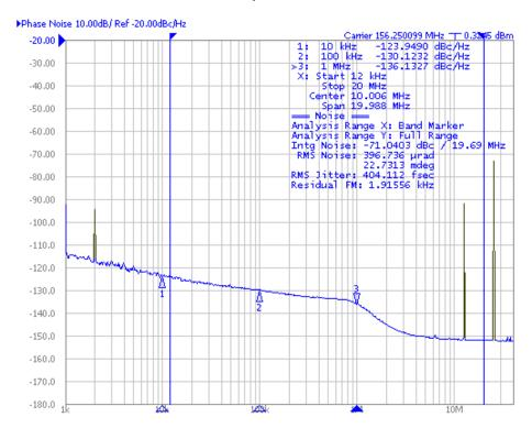
Adding one output at 100MHz causes a 12.5MHz spur but this spur is below -90dBc and does not contribute significantly to the 12K~20M phase jitter. Phase Noise levels at 10KHz, 100KHz and 1MHz are unaffected. This combination is perfect for the 5P49V6913 with two differential outputs.
