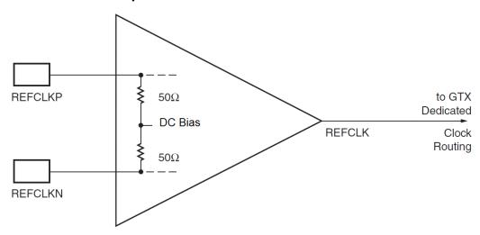
The reference clock input on the Xilinx FPGA has on-chip  $100\Omega$  ( $50\Omega + 50\Omega$ ) differential termination. The center tab between the two  $50\Omega$  resistors is biased internally and Xilinx recommends to AC couple the differential reference clock with typical 100nF capacitors to the REFCLKP and REFCLKN input pair.
