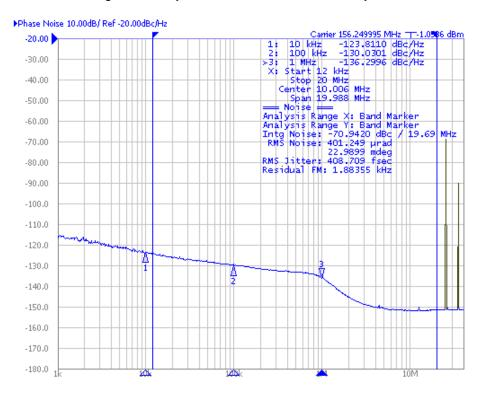
Example A2: 312.5MHz LVDS clock, generated by VersaClock 6 with a 31.25MHz crystal
