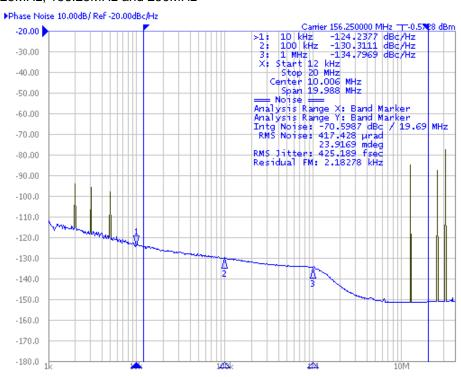
In this case the 12.5MHz spur is a little bit stronger, causing the phase jitter to increase to 425fs. Phase Noise levels at 10KHz, 100KHz and 1MHz are still unaffected. This combination is perfect for the 5P49V6901 with four differential outputs.
