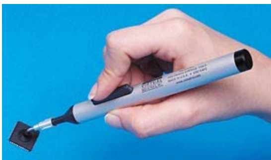
Figure 8. Manual Handling of WLCSP Device Using a Vacuum Pen
