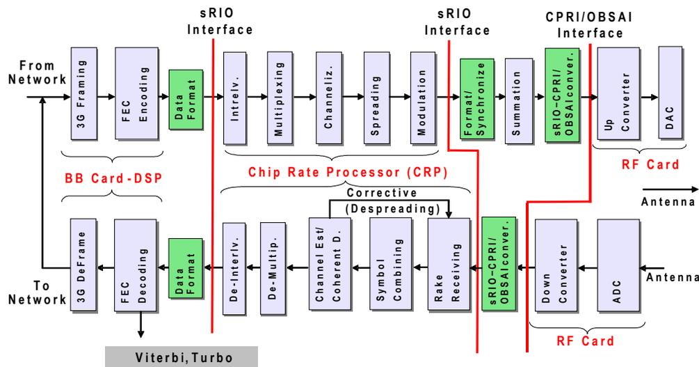
Figure 3: Algorithm-protocol partitioning for CDMA based systems
