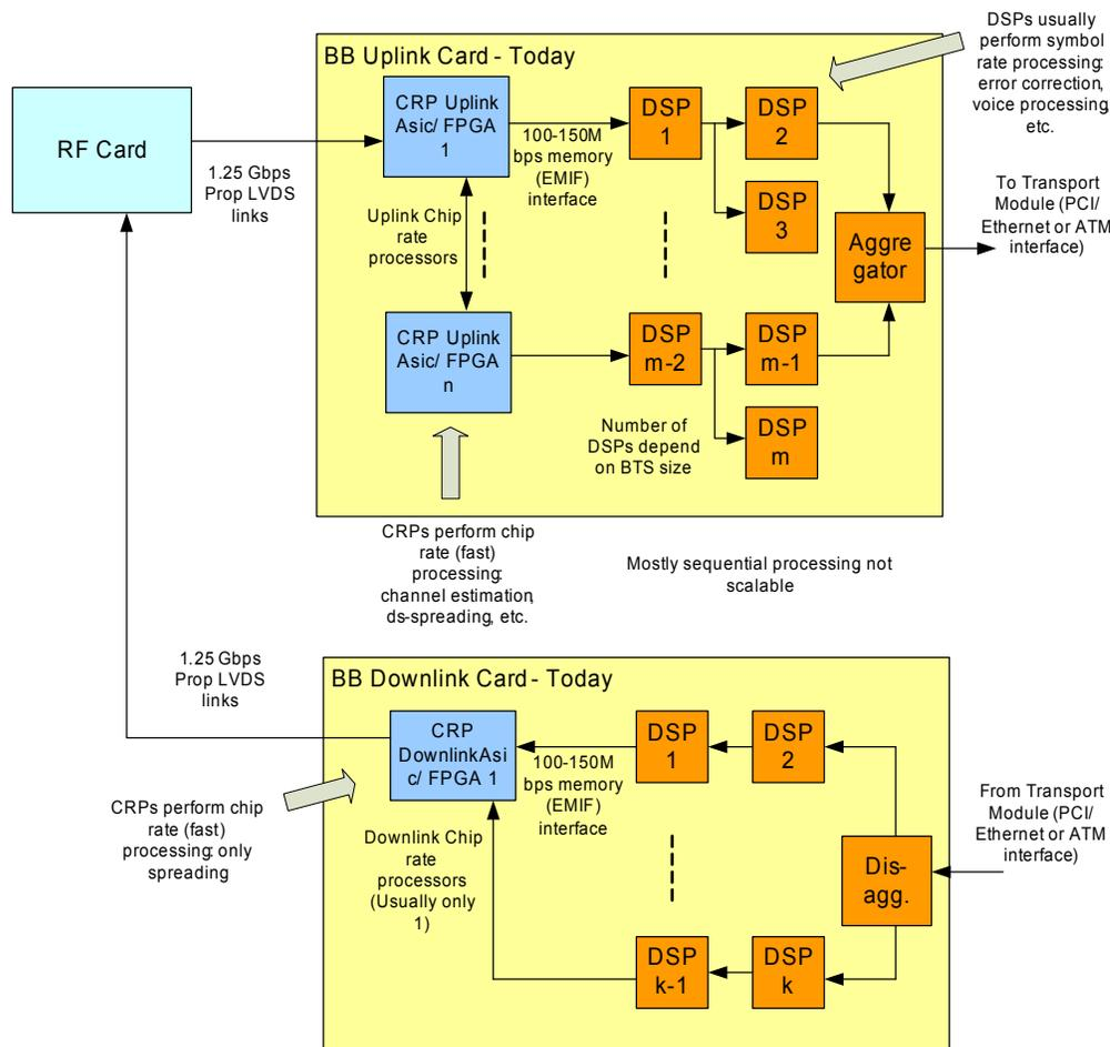
Figure 2: Today's typical base band card architecture
