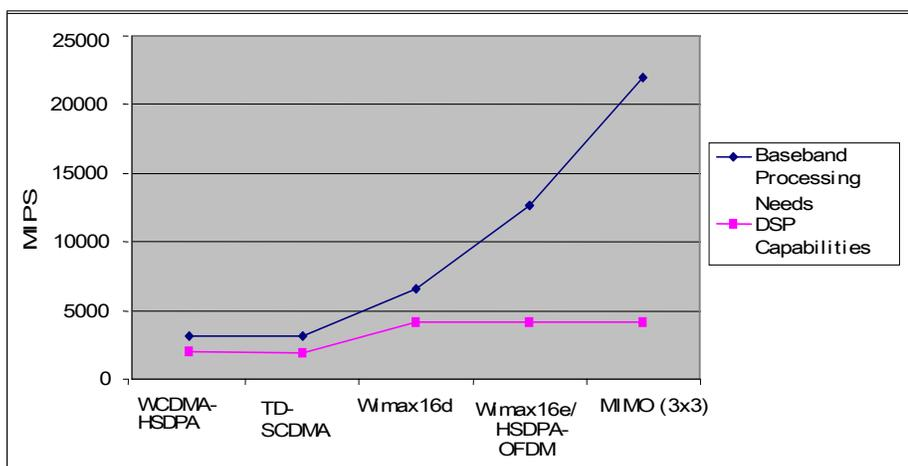
Figure 1: MIPS requirements for different wireless protocols
