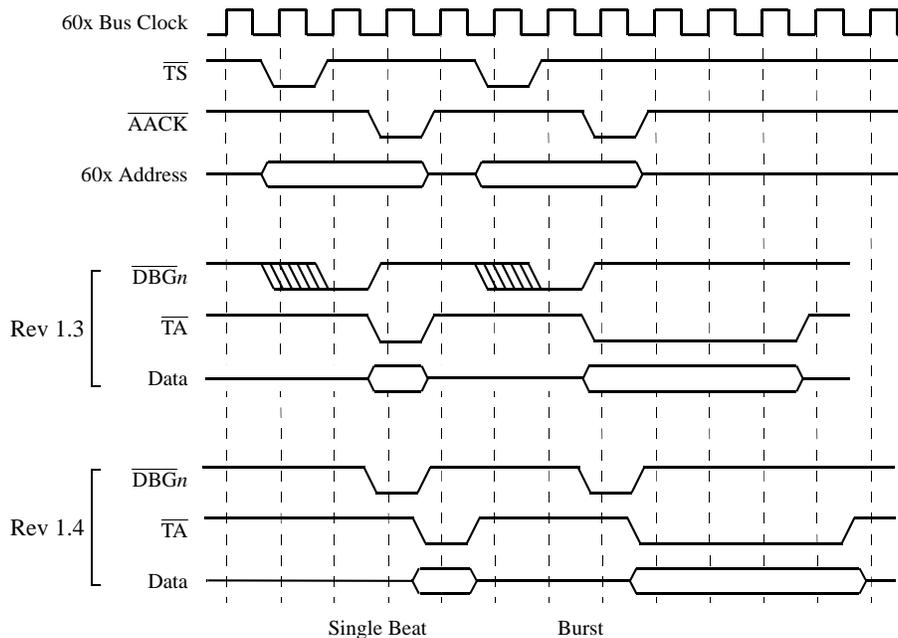
Figure 1. Rev 1.3 and Rev 1.4  $\overline{DBGn}$  Signal Timing
