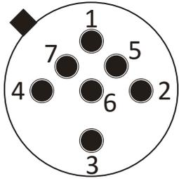
**Table 5. Pin Assignments: TO-39 Sensor Socket for SGAS707 (SEN1)**
