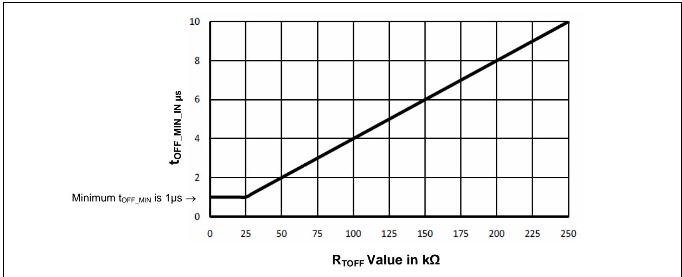
Figure 2.5 Minimum Off-Time t_{OFF\_MIN} vs. R_{TOFF}
