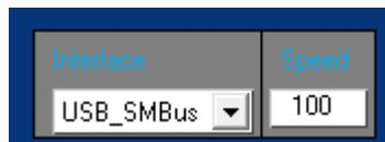
Only USB to SMBus is available, you can change the SMBus speed, but please note that the speed of SMBus is from 10KHz to 100KHz.
