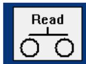
Pressing the read button will initiate a read. If a chipset is used for reading, the byte count is determined by the value in the device byte count register. The byte count cannot be larger than 32 dec. Non-read locations in the read grid will be grayed out.
