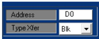
The address is 7-bit slave address combined with 0 in LSB, for example if the slave address is 1101000, D0 should be filled.
