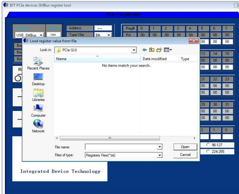
To Write register from file, click "Write Register File to Device" button, it will pop up a window, select the file path and the file name, then click "Open", the GUI will read all registers' value from the file then down load to device.
