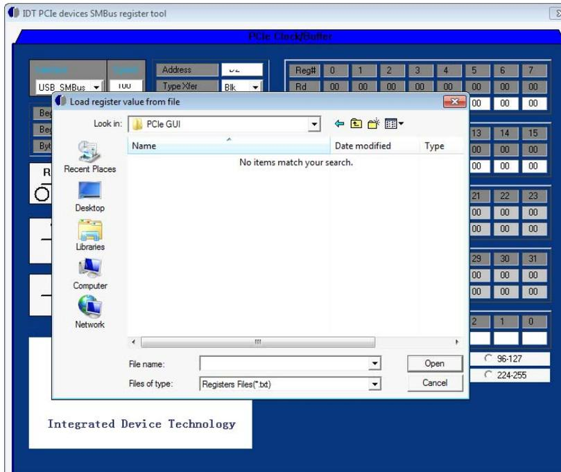
To Write register from file, click "Write Register File to Device" button, it will pop up a window, select the file path and the file name, then click "Open", the GUI will read all registers' value from the file then down load to device.
