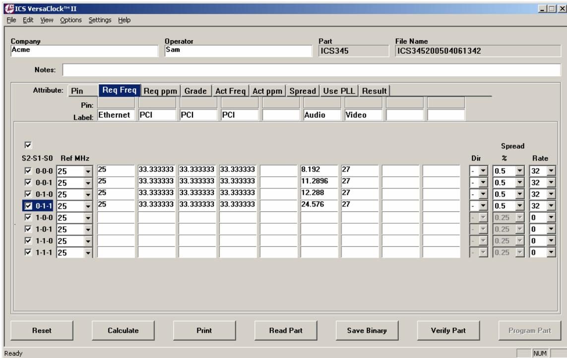
The Register that is being modified and the Attribute that is active will be highlighted. This allows you to focus on the proper information to be entered. Make sure that the entries for each Attribute aligns in the matrix with the target frequency.
