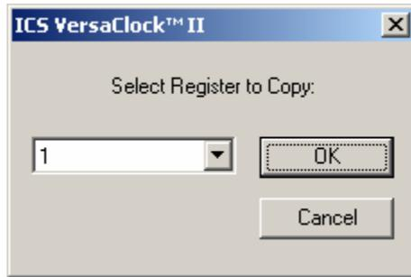
The pull down menu allows the copying of any register to the target register. You do not need to go in any specific order.
