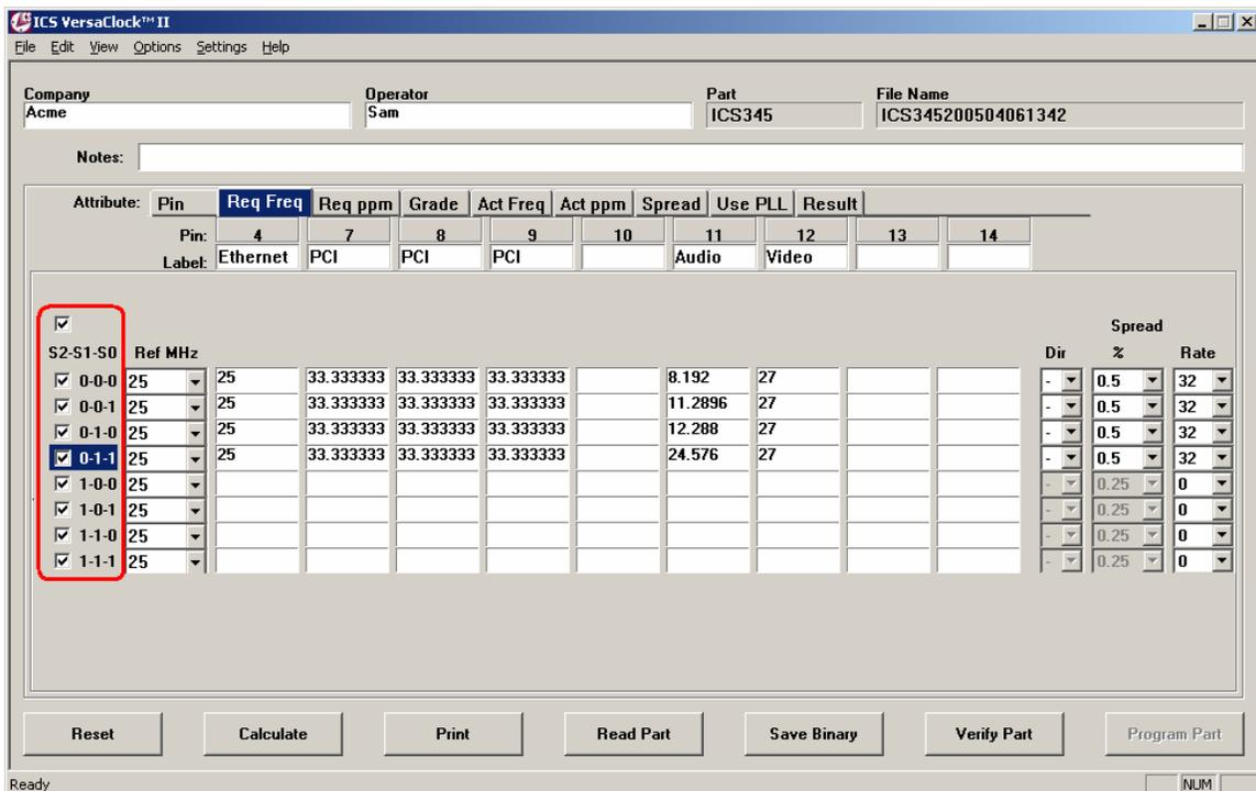
One or multiple registers can be Reset and Recalculated.
