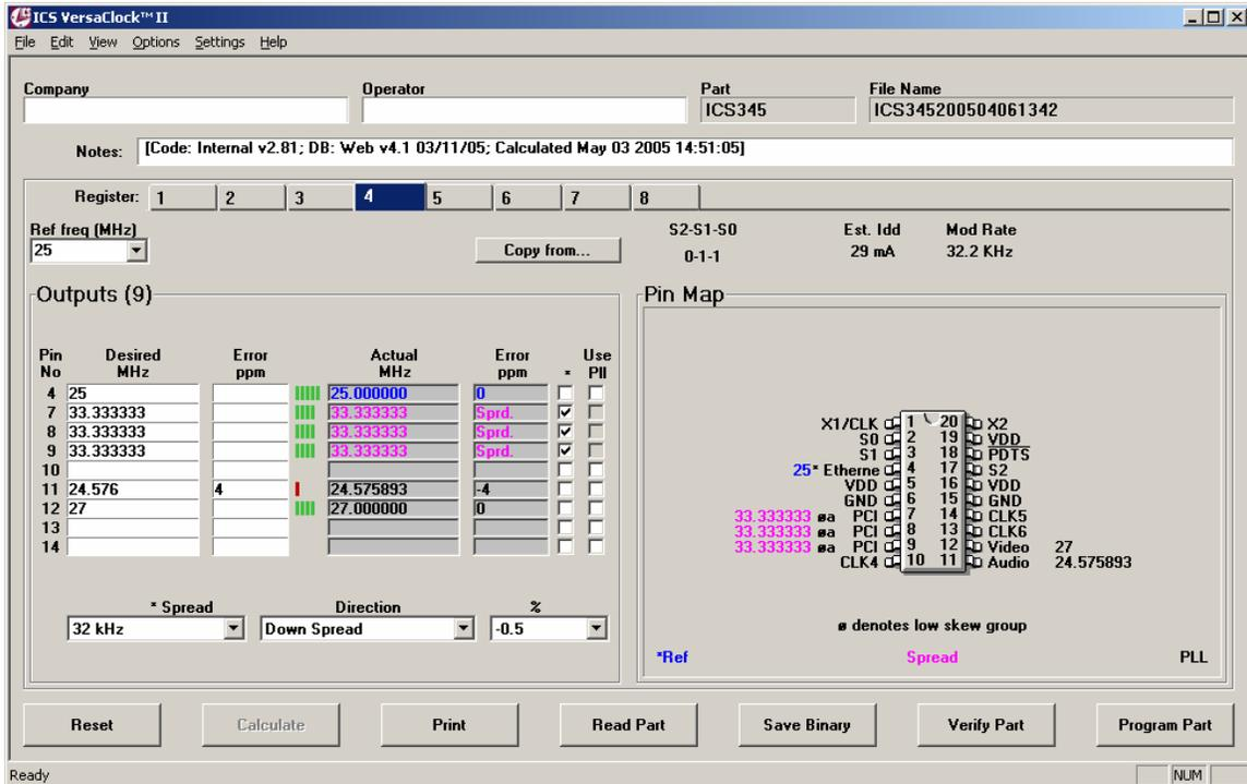
Recalculation, provided a solution with -4 ppm synthesis offset.
