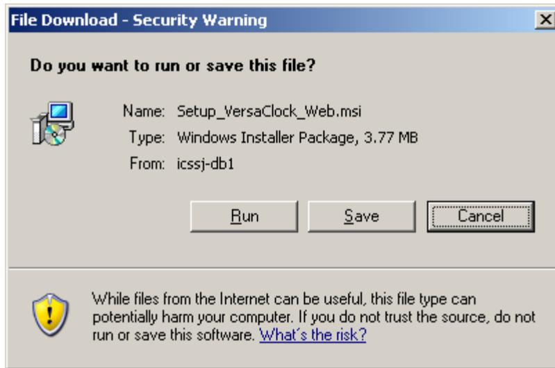
Select Run to automatically initiate the installation process and install over older versions of the software if defaults settings are used.
