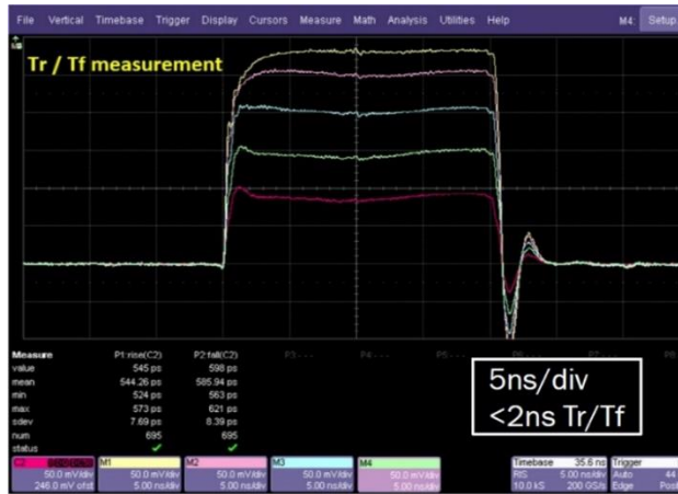
Figure 6. ISL78365 laser diode driver showing overshoot compensated pulse
