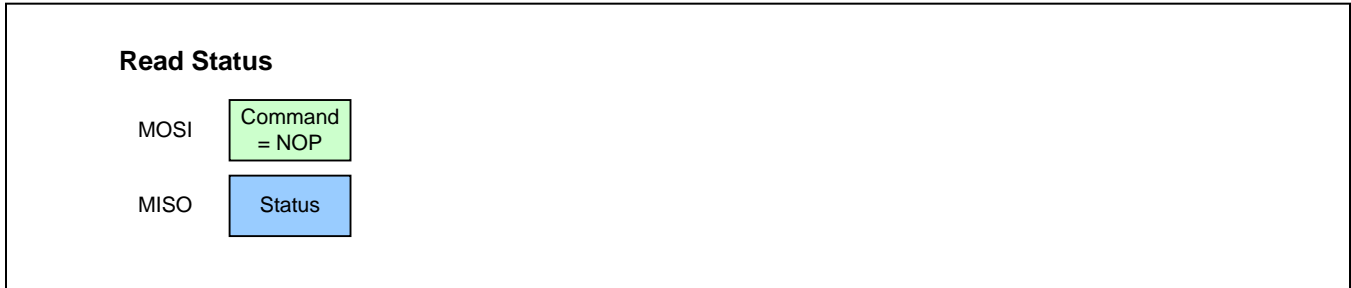
Figure 3.6 SPI Read Status
